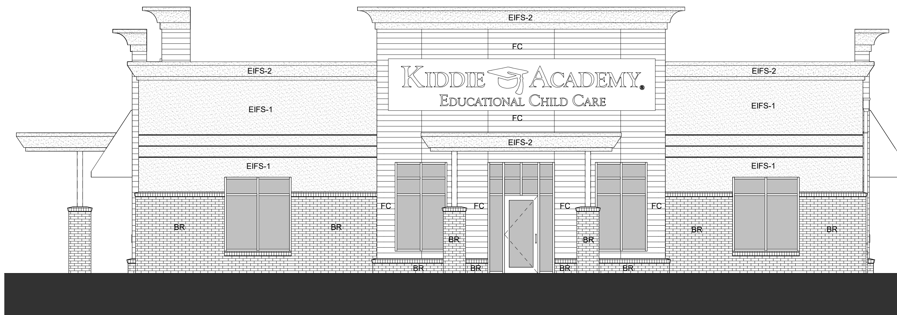
3 MCKNIGHT DRIVE ELEVATION SCALE: 3/16" = 1'-0"
