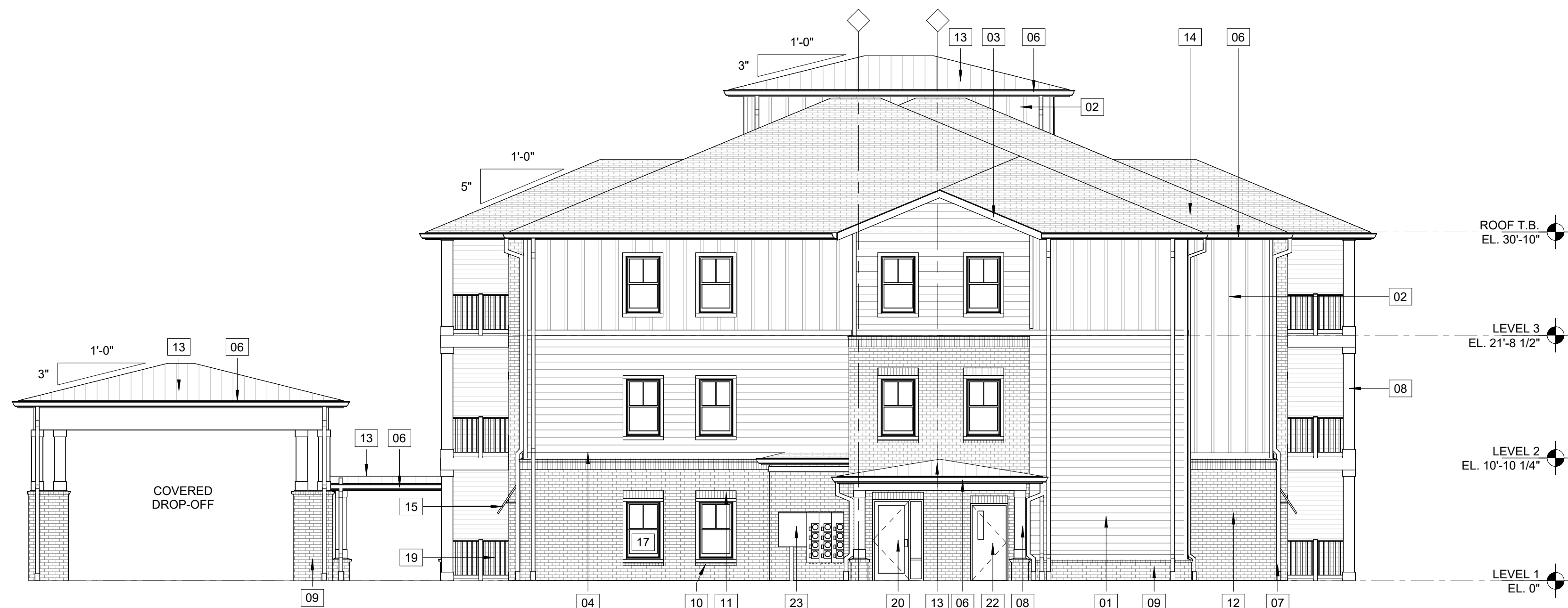
1 EXTERIOR ELEVATION (BUILDING TYPE "II") A106 | A303 1/8" = 1'-0"
