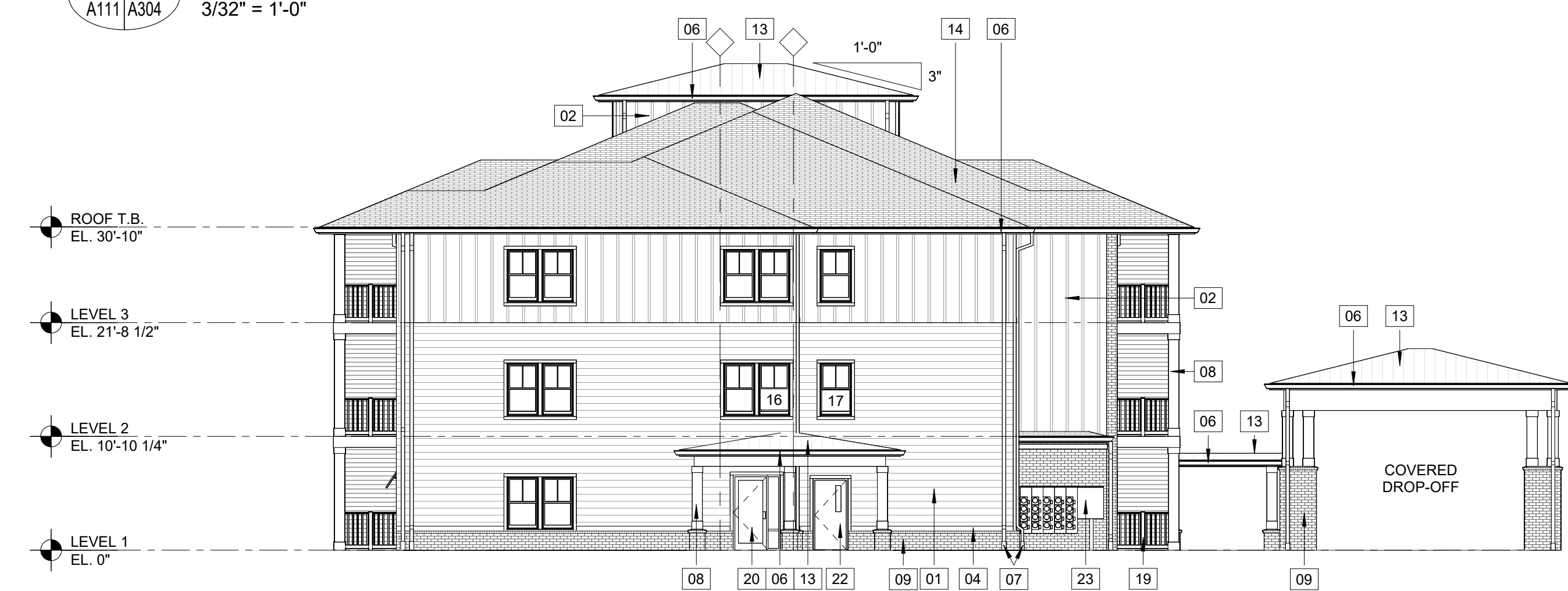
3 EXTERIOR ELEVATION (BUILDING TYPE "III") A111|A304 3/32" = 1'-0"
