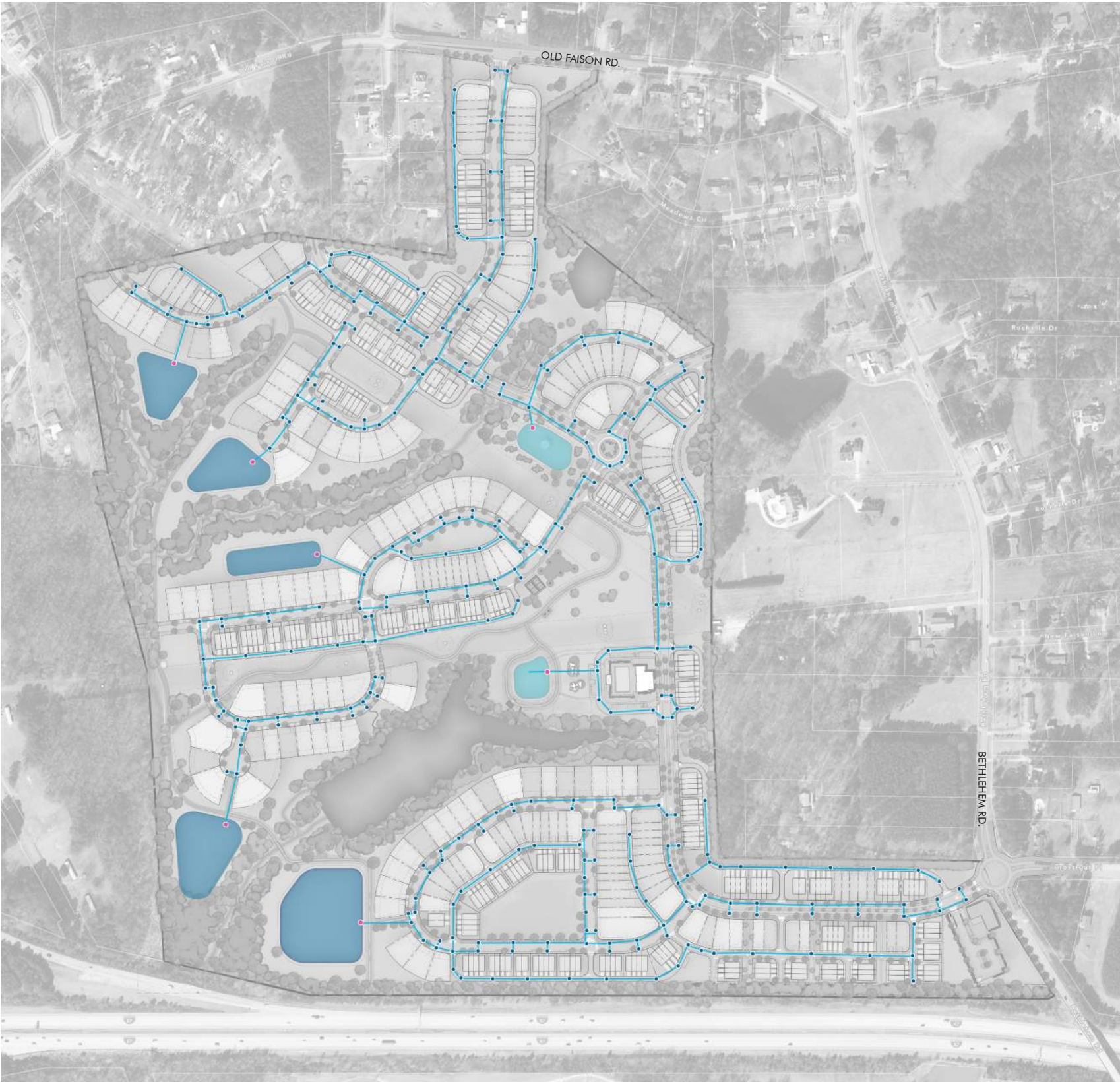
Figure 17a: Stormwater Plan for Lyndon Oaks
