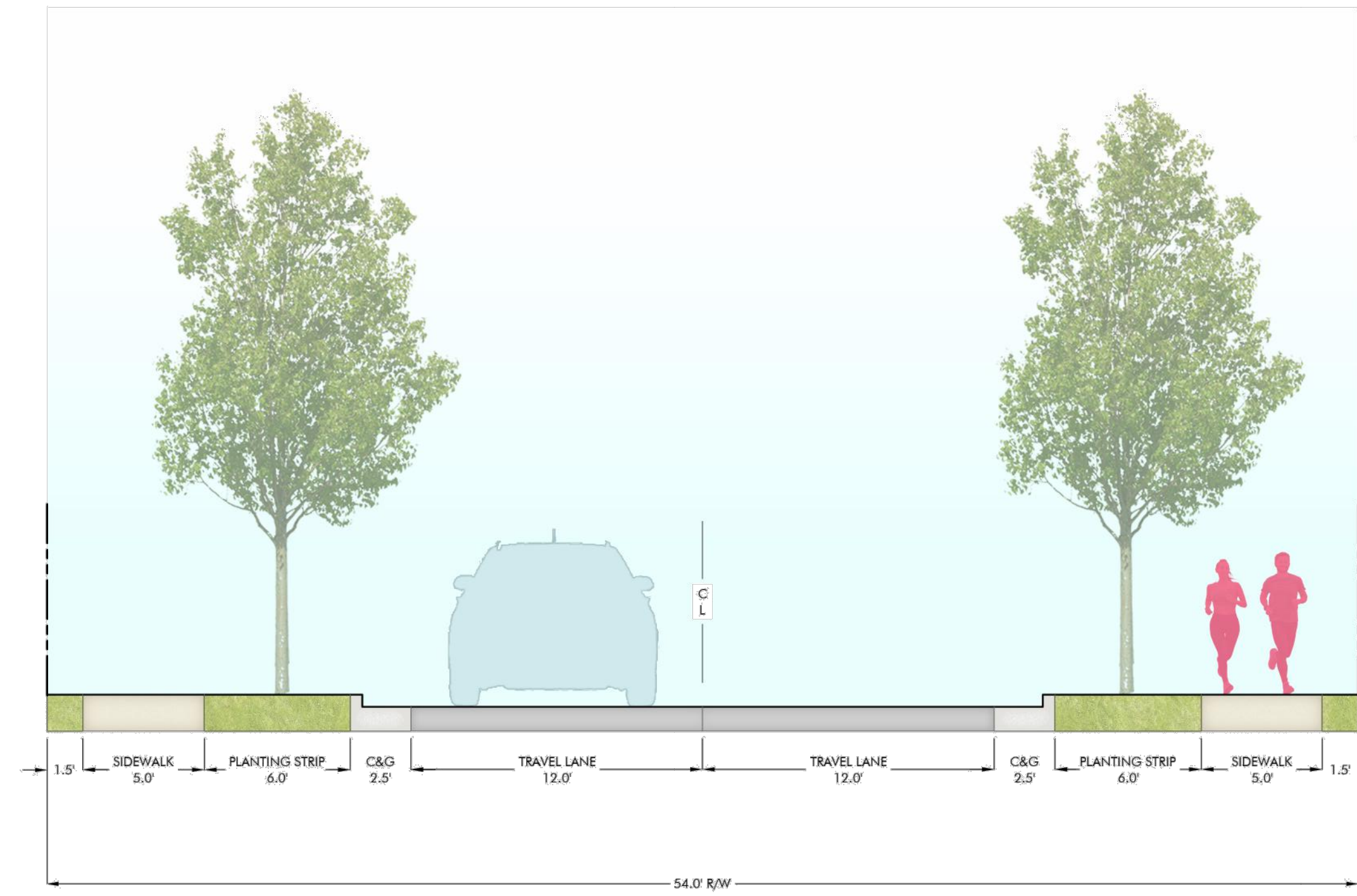
LOCAL STREET PARKING - NO ON STREET PARKING SCALE: 1" = 5'-0" SECTION
