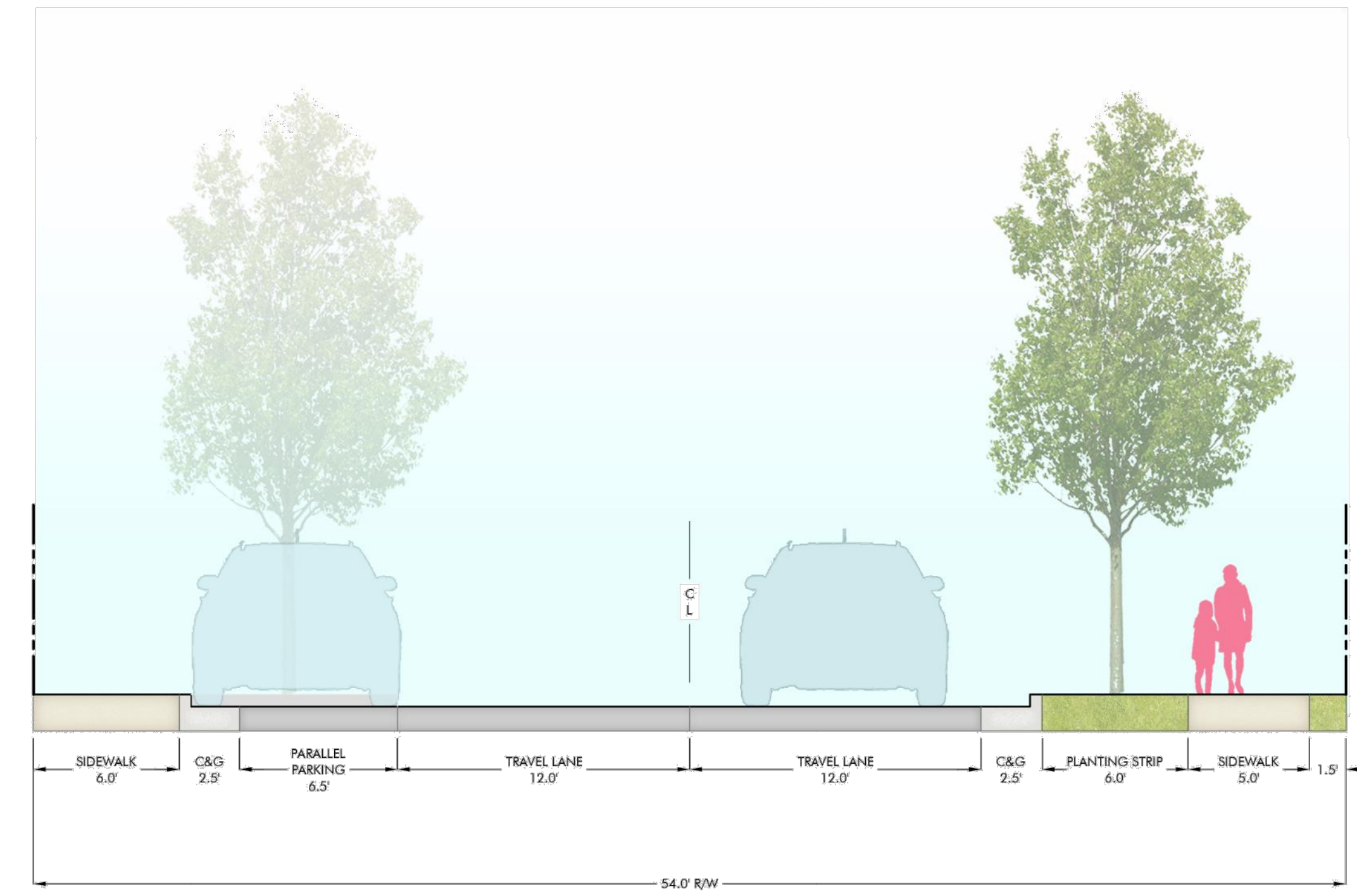
LOCAL STREET PARKING - 1 SIDE ON STREET PARKING SCALE: 1" = 5'-0" SECTION
