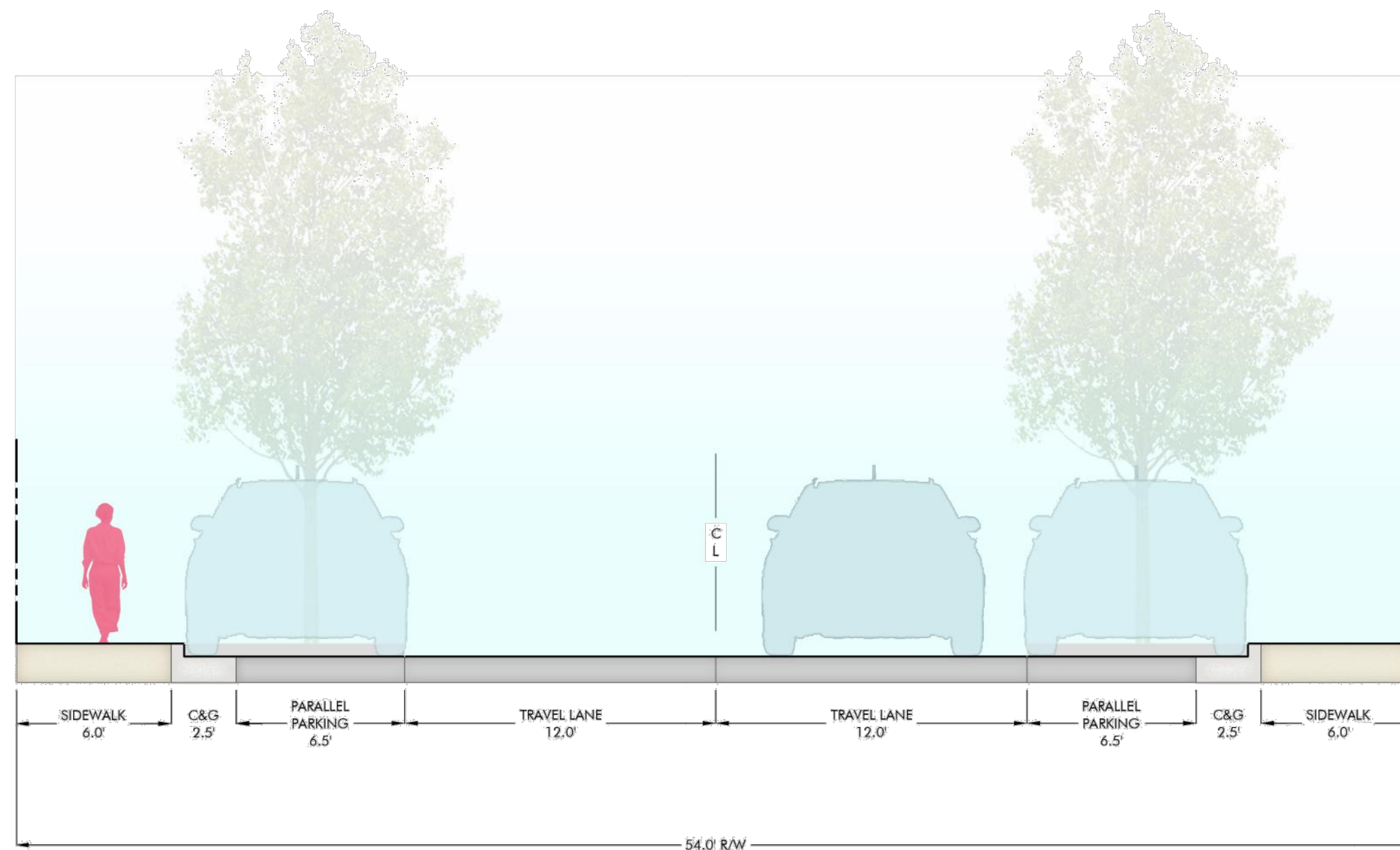
LOCAL STREET PARKING - 2 SIDE ON STREET PARKING SCALE: 1" = 5'-0" SECTION
