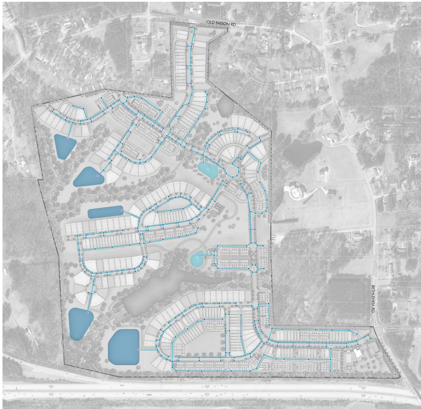
Figure 16a: Stormwater Plan for Lyndon Oaks
