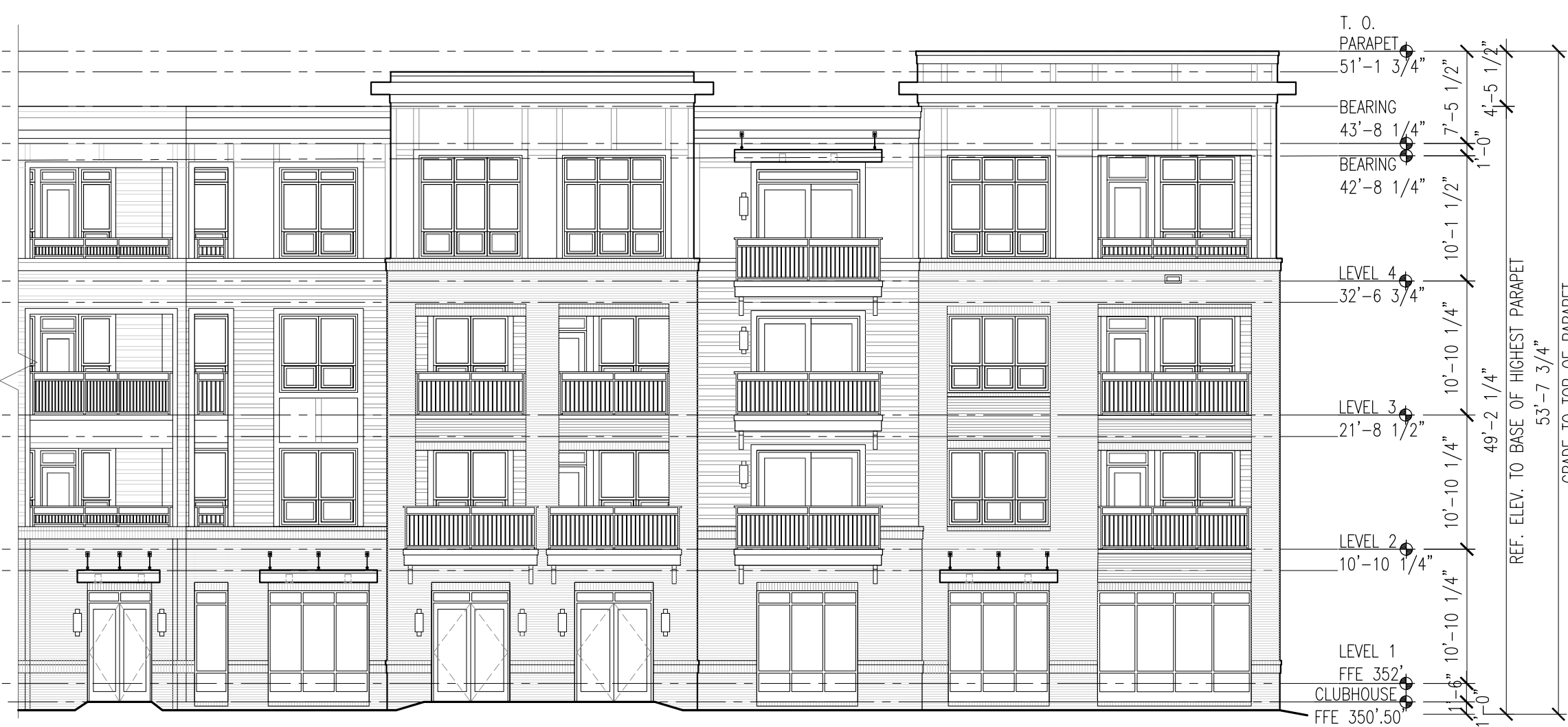
BUILDING 1: NORTH COURTYARD ELEVATION SCALE: 3/32" = 1'-0"
