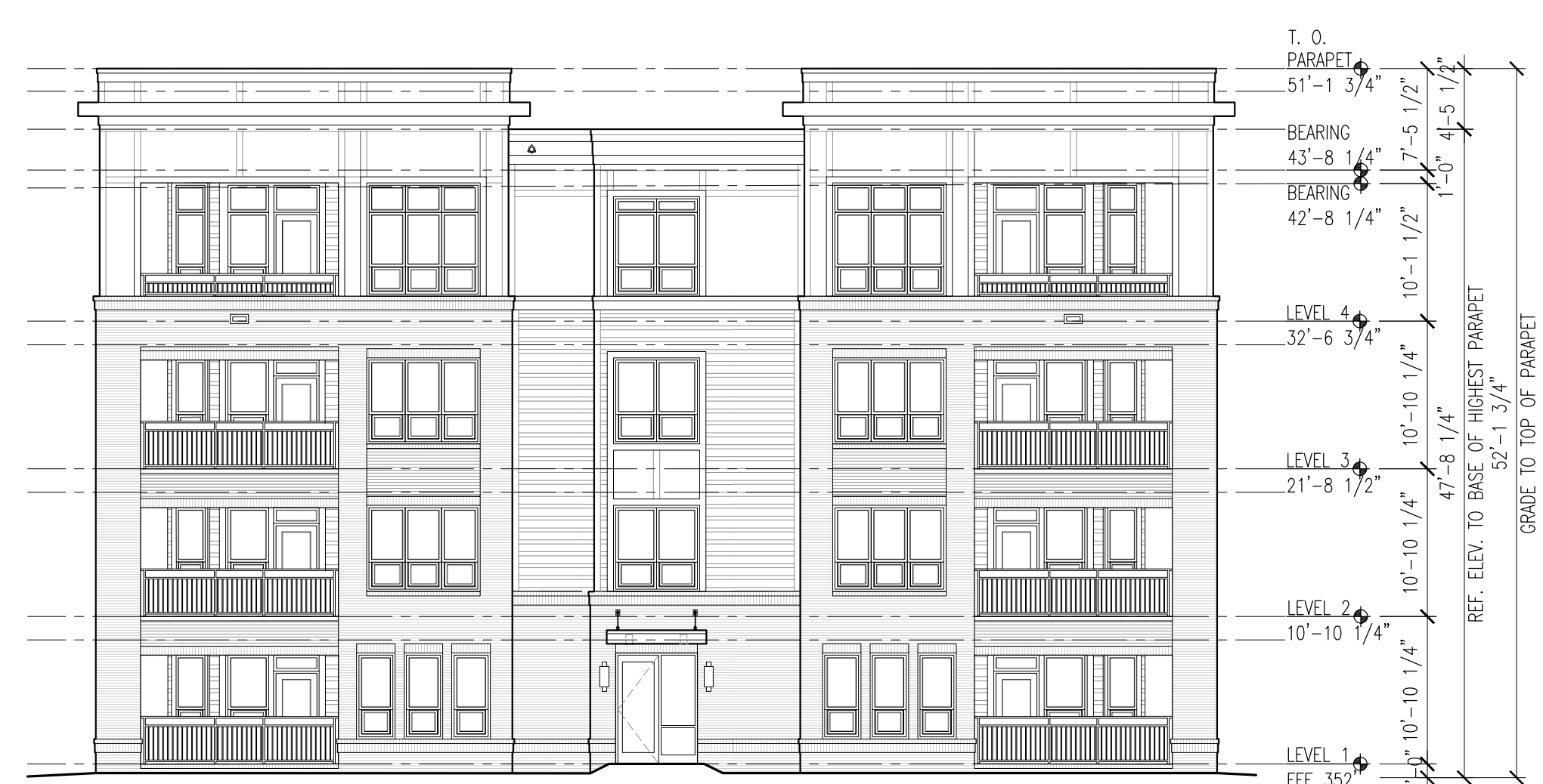
BUILDING 2: SOUTH ELEVATION SCALE: 3/32" = 1'-0"
