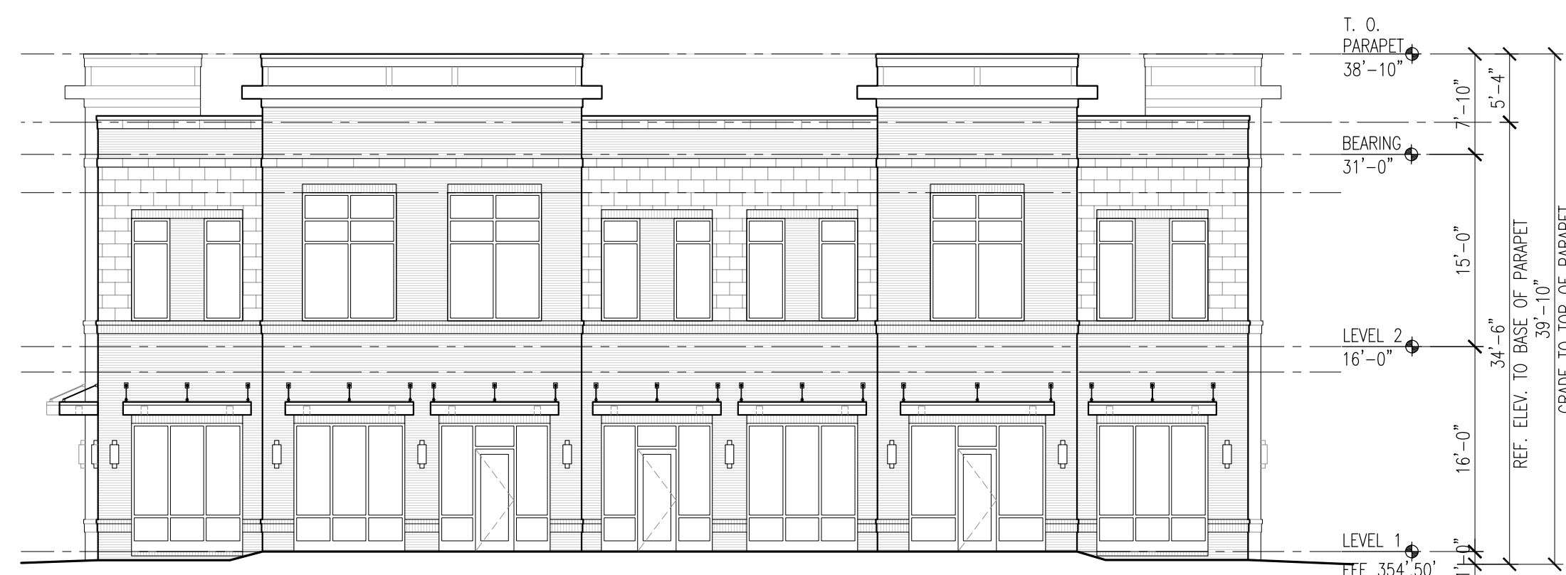
BUILDING 3: SOUTH ELEVATION SCALE: 3/32" = 1'-0"
