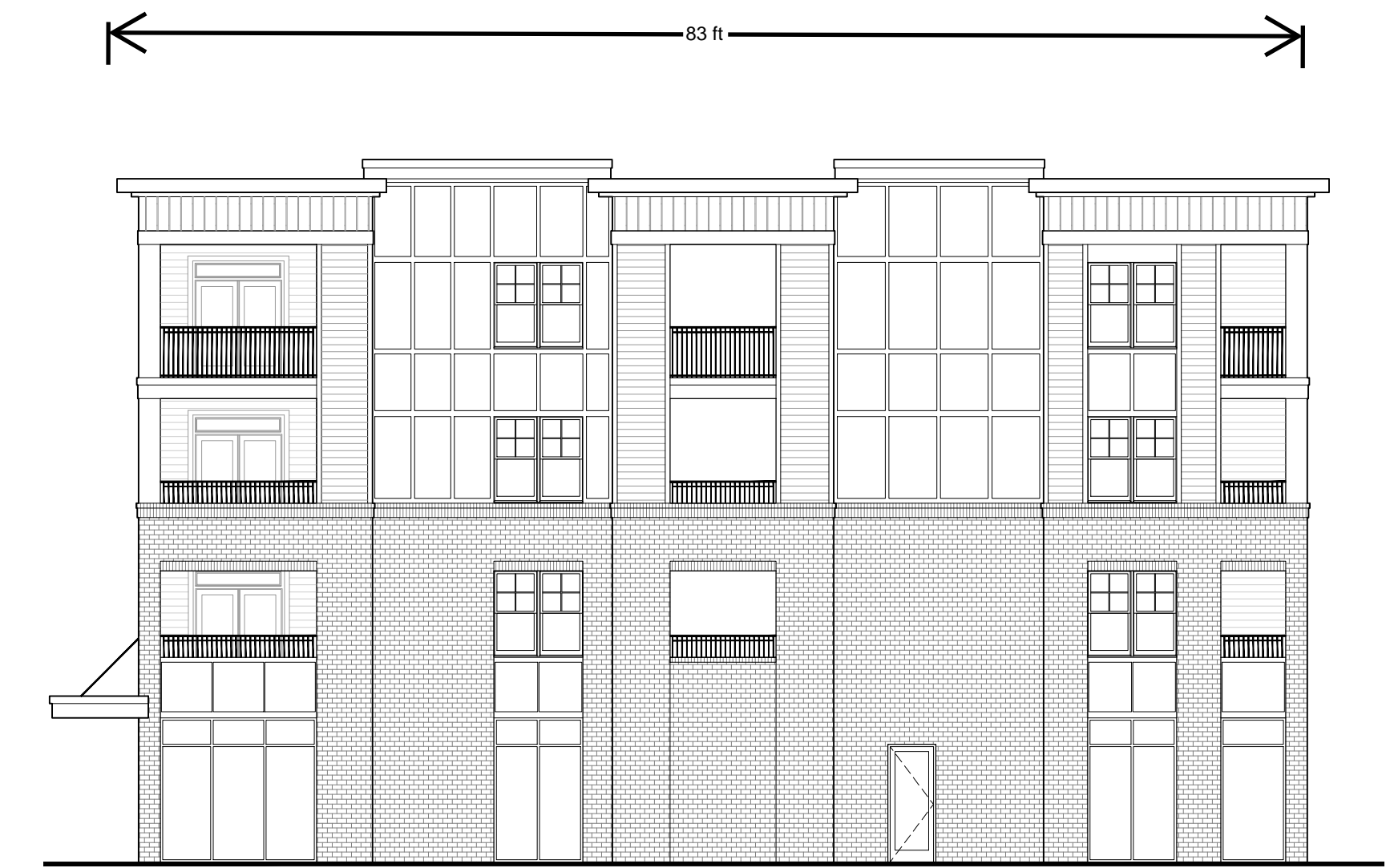
2 BUILDING 1 - EAST / WEST ELEVATION Scale: 3/32" = 1'-0"
