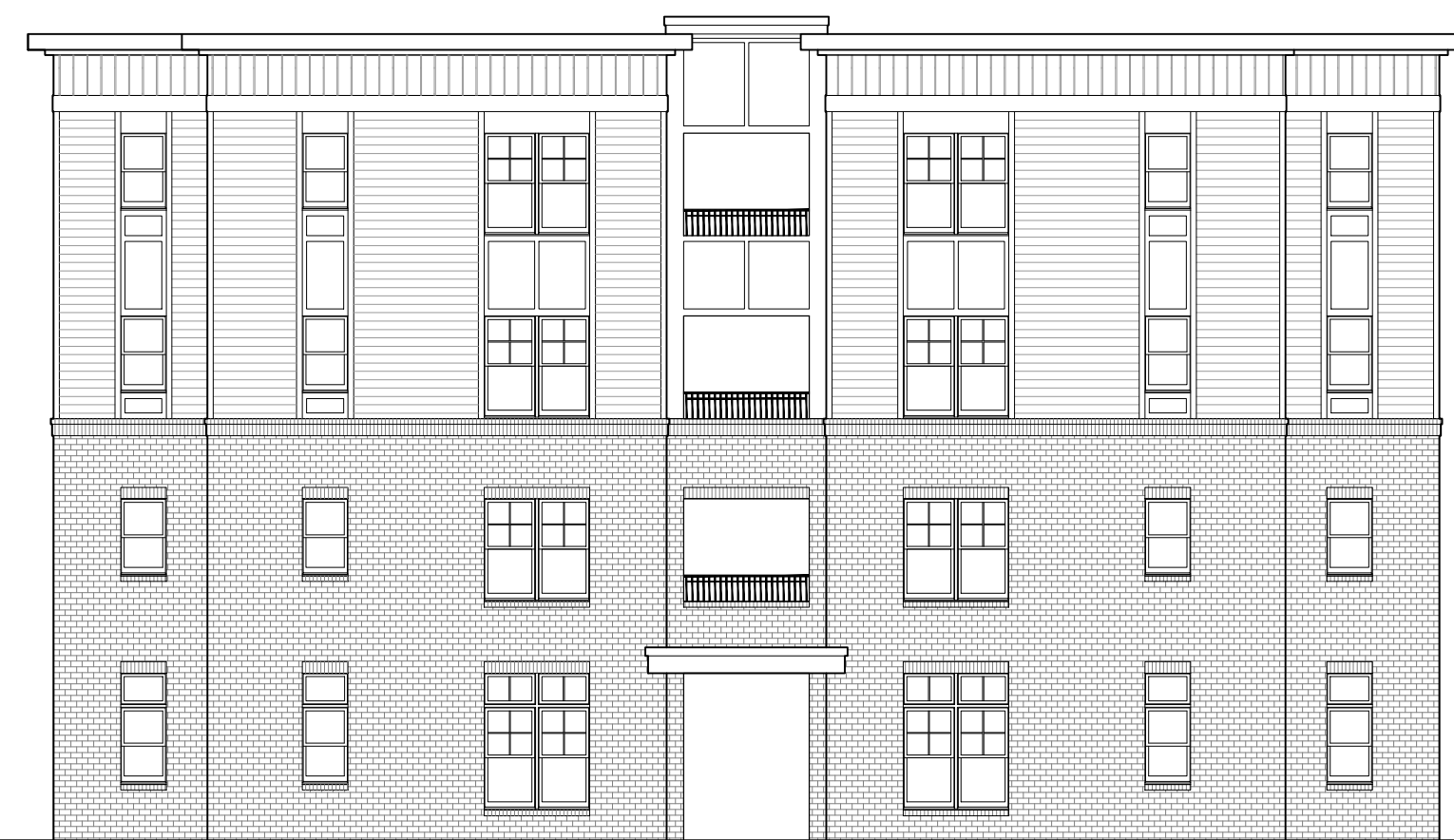
3 BUILDING 5 - END ELEVATION Scale: 3/32" = 1'-0"
