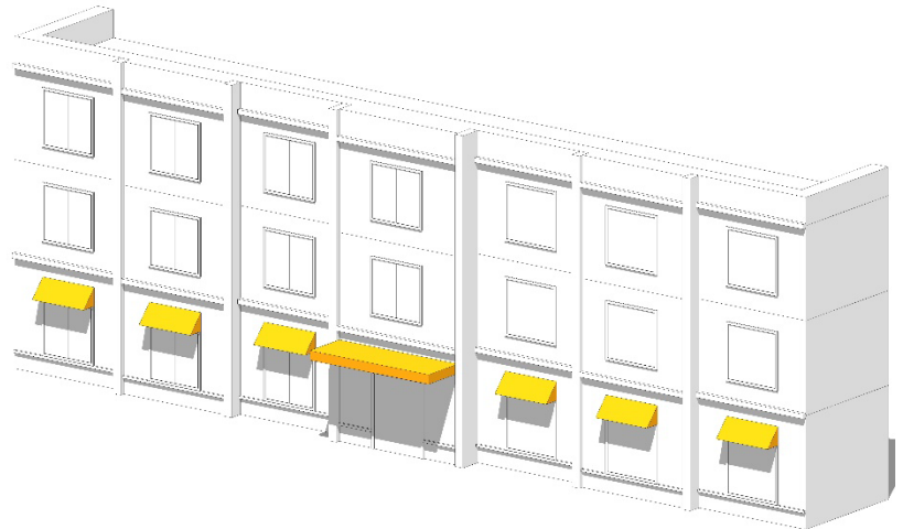
Figure 6.22. Mixed Use Building Type Awnings
