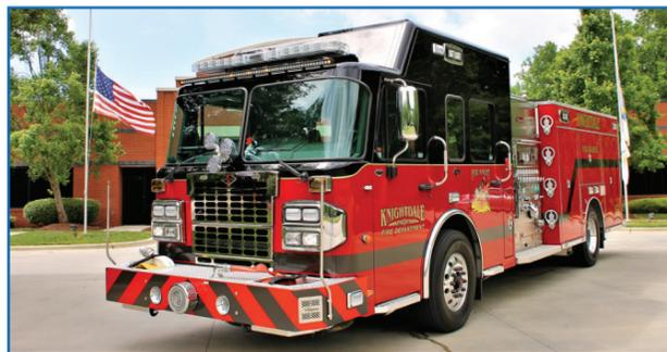
all LED lighting package including a light bar on the front of the cab that allows for more on-scene lighting visibility. It has more compartment space to hold additional equipment for the variety of calls our department runs, from fire suppression to rescue and medical calls.
