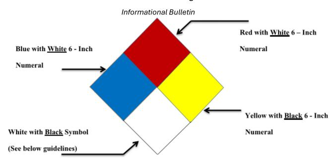
This placard is representative of the general hazards of chemicals or materials that may be stored in a building or room, and is used to alert emergency responding personnel of the type and degree of hazard, based on the criteria indicated below.
