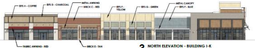
3 NORTH ELEVATION - BUILDING I-K 1/16" = 1'-0" GLAZING CALCULATIONS: 325' X 14'6" = 4,733 SF X 0.4 = 1,893 SF REQUIRED (40%) ACTUAL GLAZING PROVIDED: 1,730 SF (50%)
