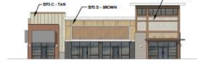
10 NORTHEAST ELEVATION - BUILDING E 1/16" = 1'-0" GLAZING CALCULATIONS: 361' X 14'6" = 525 SF X 0.4 = 210 SF REQUIRED (40%) ACTUAL GLAZING PROVIDED: 410 SF (21%)
