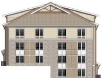
7 SIDE ELEVATION - TYPICAL 28 UNIT APARTMENT BUILDING - 3 BR 1/16" = 1'-0"
