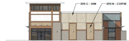
3 NORTH ELEVATION - BUILDING B 1/16" = 1'-0" GLAZING CALCULATIONS: 72'L X 14'H = 1,008 SF X 0.4 = 403 SF REQUIRED (40%) ACTUAL GLAZING PROVIDED: 264 SF (26%)
