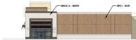
4 SOUTH ELEVATION - BUILDING G-H 1/16" = 1'-0" GLAZING CALCULATIONS: 100' X 14'6" = 1,456 SF X 0.4 = 582 SF REQUIRED (40%) ACTUAL GLAZING PROVIDED: 190 SF (14%)
