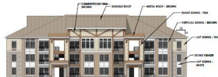
1 FRONT ELEVATION - TYPICAL 24 UNIT APARTMENT BUILDING - 3 BR 1/16" = 1'-0"
