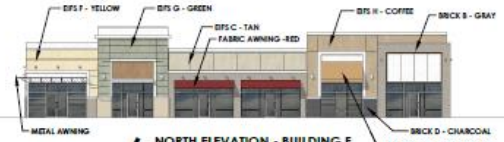
6 NORTH ELEVATION - BUILDING F 1/16" = 1'-0" GLAZING CALCULATIONS: 130' X 14'6" = 1,878 SF X 0.4 = 751 SF REQUIRED (40%) ACTUAL GLAZING PROVIDED: 890 SF (27%)
