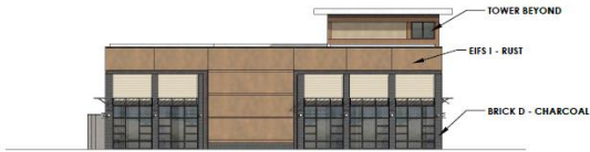
2 SOUTH ELEVATION - BUILDING B 1/16" = 1'-0" GLAZING CALCULATIONS: 75'L X 14'H = 1,050 SF X 0.4 = 420 SF REQUIRED (40%) ACTUAL GLAZING PROVIDED: 430 SF (41%)
