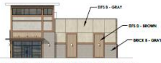
12 NORTHWEST ELEVATION - BUILDING E 1/16" = 1'-0" GLAZING CALCULATIONS: 401' X 14'6" = 582 SF X 0.4 = 233 SF REQUIRED (40%) ACTUAL GLAZING PROVIDED: 140 SF (19%)
