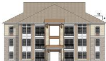
3 FRONT ELEVATION - TYPICAL 12 UNIT APARTMENT BUILDING - 3 BR 1/16" = 1'-0"
