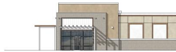
7 EAST ELEVATION - BUILDING A 1/16" = 1'-0" GLAZING CALCULATIONS: 60'L X 14'H = 840 SF X 0.4 = 336 SF REQUIRED (40%) ACTUAL GLAZING PROVIDED: 160 SF (19%)
