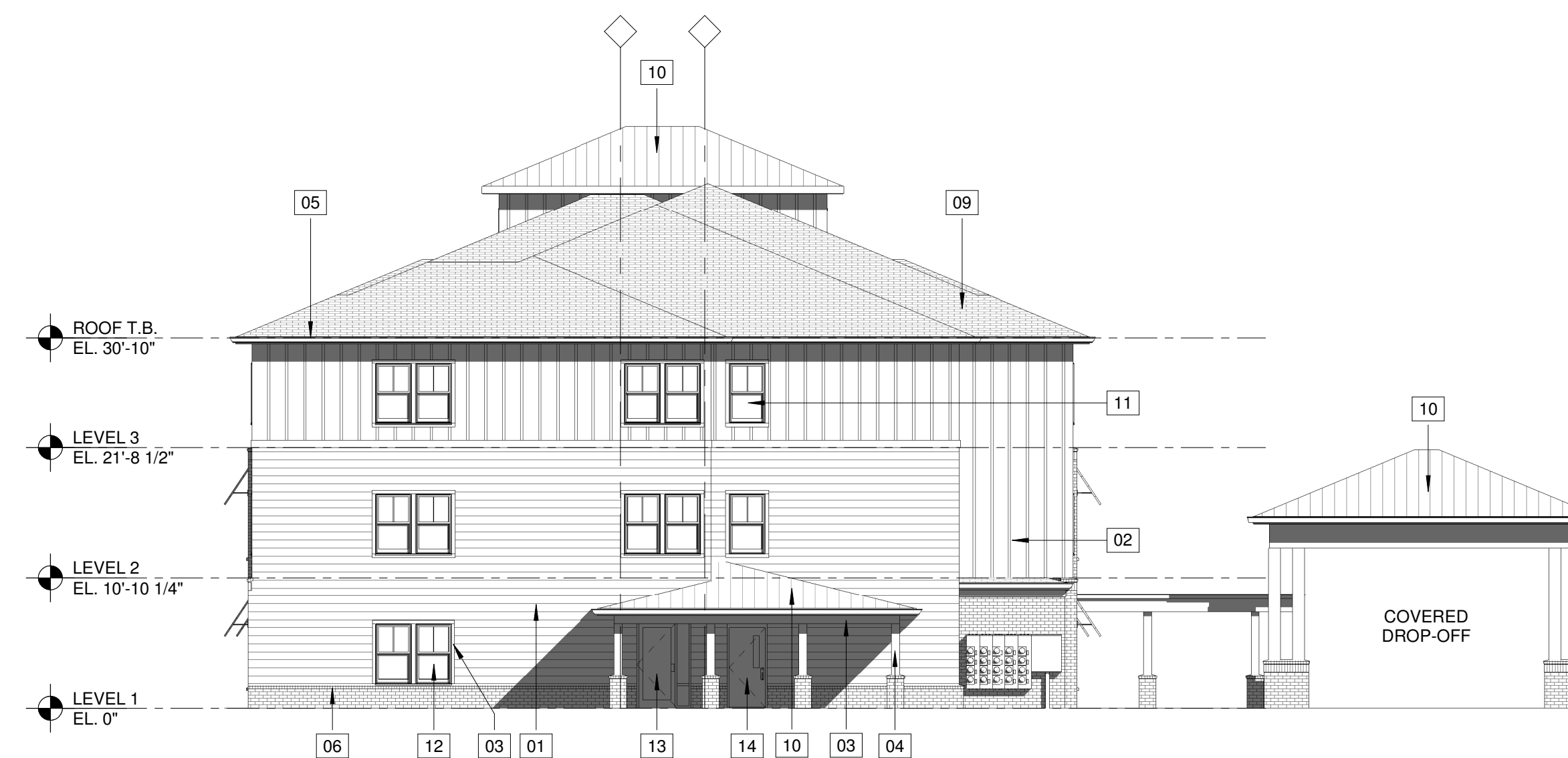
2 EXTERIOR ELEVATIONS (BUILDING TYPE "II") A107 | A304 3/32" = 1'-0"
