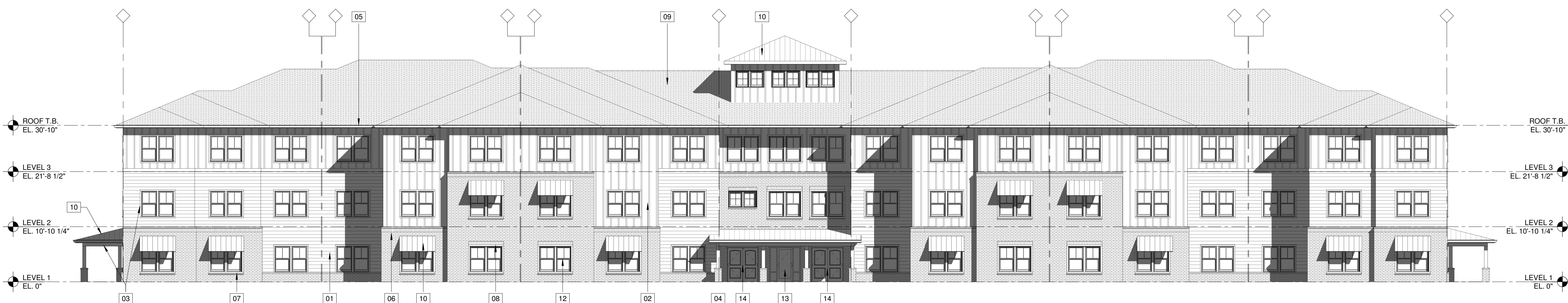
2 EXTERIOR ELEVATIONS (BUILDING TYPE "II") A107/A303 3/32" = 1'-0"
