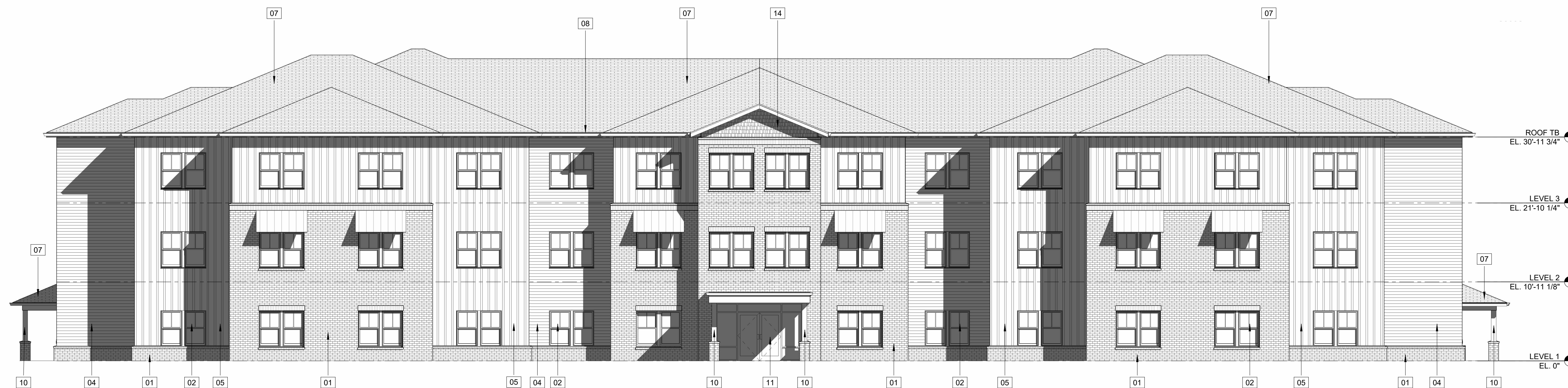
1 EXTERIOR BUILDING ELEVATION A301 1/8" = 1'-0"
