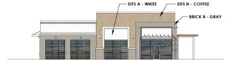
5 SOUTH ELEVATION - BUILDING A 1/16" = 1'-0" GLAZING CALCULATIONS: 69'L X 14'H = 966 SF X 0.4 = 386 SF REQUIRED (40%) ACTUAL GLAZING PROVIDED: 480 SF (50%)
