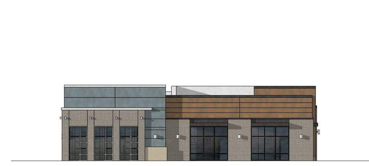
8 WEST ELEVATION - BUILDING C 1/16" = 1'-0" GLAZING CALCULATIONS: 70'L X 14'H = 980 SF X 0.4 = 392 SF REQUIRED (40%) ACTUAL GLAZING PROVIDED: 370 SF (38%)
