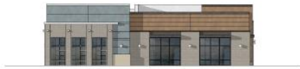
8 WEST ELEVATION - BUILDING C 1/16" = 1'-0" GLAZING CALCULATIONS: 70'L X 14'H = 980 SF X 0.4 = 392 SF REQUIRED (40%) ACTUAL GLAZING PROVIDED: 370 SF (38%)
