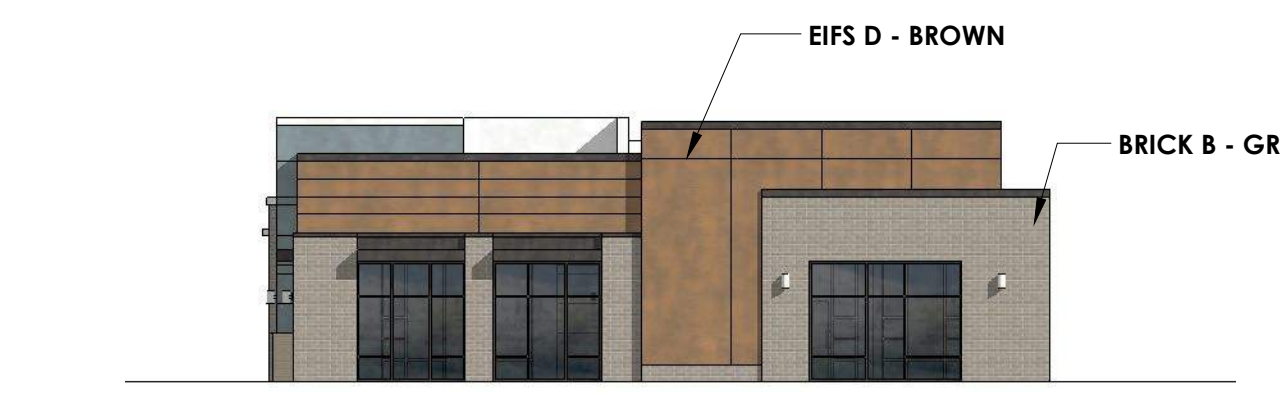
6 SOUTH ELEVATION - BUILDING C 1/16" = 1'-0" GLAZING CALCULATIONS: 58'L X 14'H = 812 SF X 0.4 = 325 SF REQUIRED (40%) ACTUAL GLAZING PROVIDED: 310 SF (38%)
