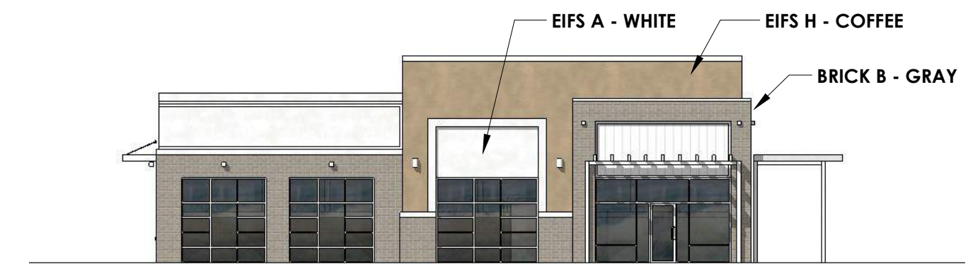
5 SOUTH ELEVATION - BUILDING A 1/16" = 1'-0" GLAZING CALCULATIONS: 49'L X 14'H = 966 SF X 0.4 = 386 SF REQUIRED (40%) ACTUAL GLAZING PROVIDED: 480 SF (50%)
