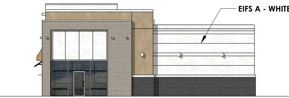
8 WEST ELEVATION - BUILDING F 1/16" = 1'-0" GLAZING CALCULATIONS: 59'L X 14'H = 826 SF X 0.4 = 330 SF REQUIRED (40%) ACTUAL GLAZING PROVIDED: 160 SF (19%)
