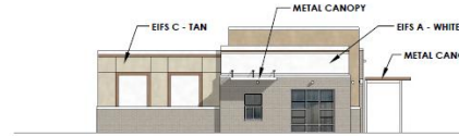
6 WEST ELEVATION - BUILDING A 1/16" = 1'-0" GLAZING CALCULATIONS: 59'L X 14'H = 826 SF X 0.4 = 330 SF REQUIRED (40%) ACTUAL GLAZING PROVIDED: 124 SF (15%)
