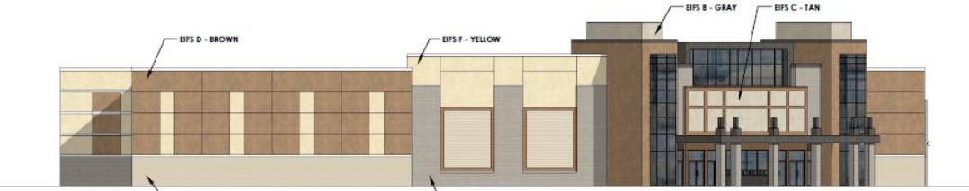
2 EAST ELEVATION - BUILDING D 1/16" = 1'-0" GLAZING CALCULATIONS: 236'L X 14'H = 3,304 SF X 0.4 = 1,322 SF REQUIRED (40%) ACTUAL GLAZING PROVIDED: 1,556 SF (47%)
