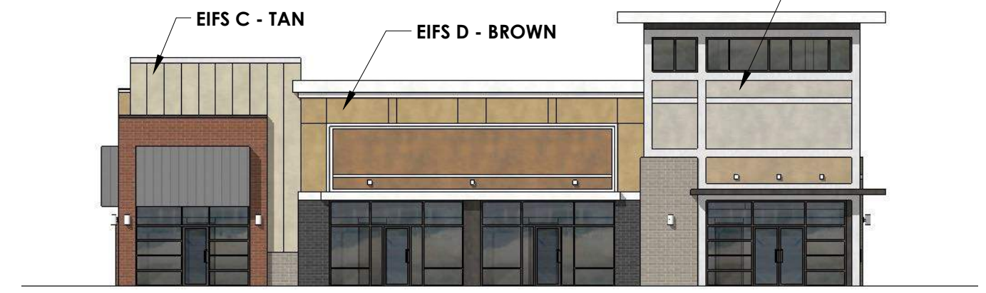
10 NORTHEAST ELEVATION - BUILDING E 1/16" = 1'-0" GLAZING CALCULATIONS: 86'L X 14'H = 1,204 SF X 0.4 = 482 SF REQUIRED (40%) ACTUAL GLAZING PROVIDED: 610 SF (51%)
