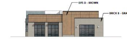
6 SOUTH ELEVATION - BUILDING C 1/16" = 1'-0" GLAZING CALCULATIONS: 58'L X 14'H = 812 SF X 0.4 = 325 SF REQUIRED (40%) ACTUAL GLAZING PROVIDED: 310 SF (38%)
