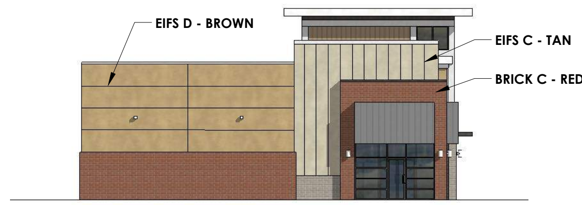
11 SOUTHEAST ELEVATION - BUILDING E 1/16" = 1'-0" GLAZING CALCULATIONS: 60'L X 14'H = 840 SF X 0.4 = 336 SF REQUIRED (40%) ACTUAL GLAZING PROVIDED: 130 SF (15%)
