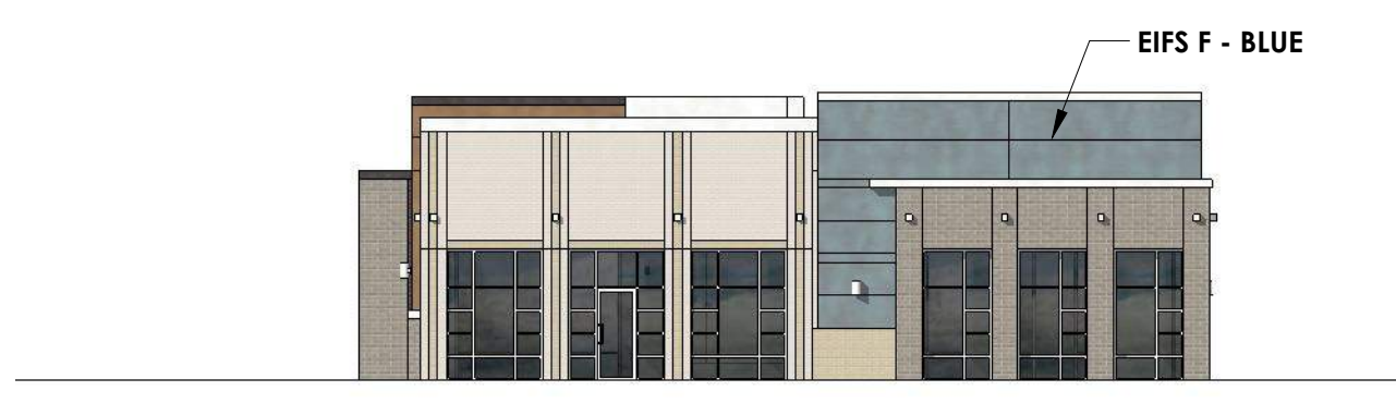
7 NORTH ELEVATION - BUILDING C 1/16" = 1'-0" GLAZING CALCULATIONS: 60'L X 14'H = 840 SF X 0.4 = 336 SF REQUIRED (40%) ACTUAL GLAZING PROVIDED: 390 SF (46%)
