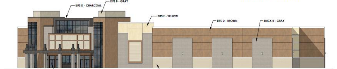
1 NORTH ELEVATION - BUILDING D 1/16" = 1'-0" GLAZING CALCULATIONS: NONE
