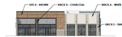
5 EAST ELEVATION - BUILDING C 1/16" = 1'-0" GLAZING CALCULATIONS: 70'L X 14'H = 980 SF X 0.4 = 392 SF REQUIRED (40%) ACTUAL GLAZING PROVIDED: 540 SF (55%)
