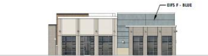
7 NORTH ELEVATION - BUILDING C 1/16" = 1'-0" GLAZING CALCULATIONS: 60'L X 14'H = 840 SF X 0.4 = 336 SF REQUIRED (40%) ACTUAL GLAZING PROVIDED: 390 SF (46%)
