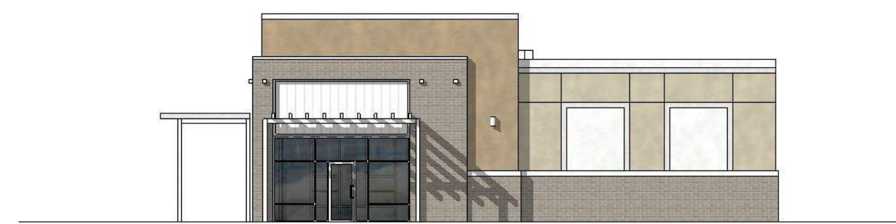
7 EAST ELEVATION - BUILDING A 1/16" = 1'-0" GLAZING CALCULATIONS: 60'L X 14'H = 840 SF X 0.4 = 336 SF REQUIRED (40%) ACTUAL GLAZING PROVIDED: 160 SF (19%)
