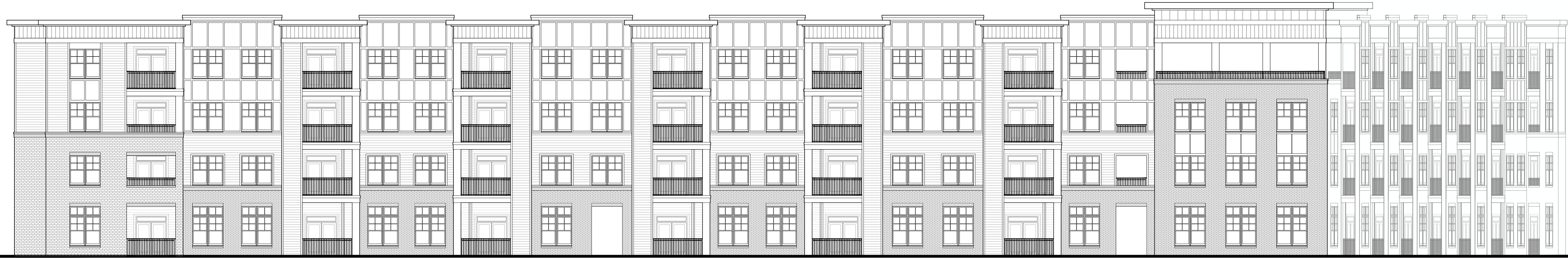
1 BUILDING 5 - NORTH ELEVATION Scale: 3/32" = 1'-0"
