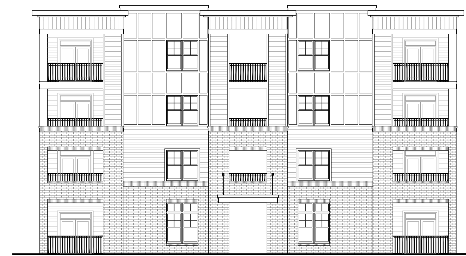
2 BUILDING 4 - EAST / WEST ELEVATION Scale: 3/32" = 1'-0"
